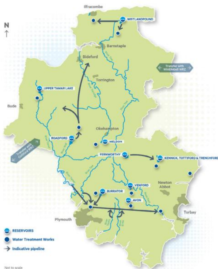
Figure 5-1 Roadford WRZ Water Supply
