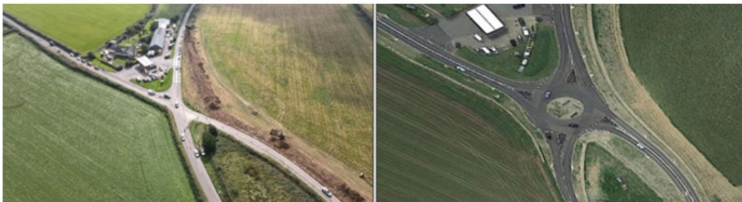
Figure 33 – Lynton Cross safety improvements, with crossroads upgraded to a roundabout.
