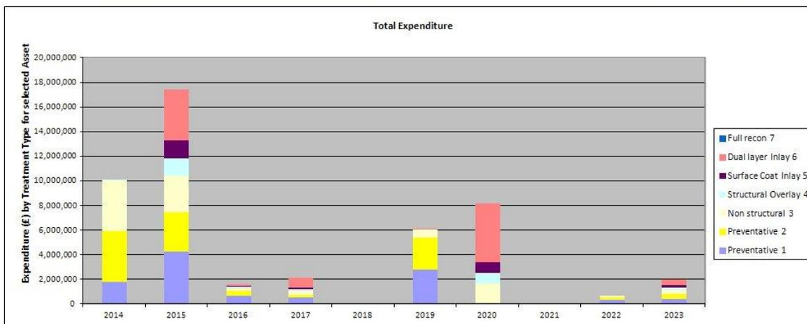
2.15 The above scenario involves a combination of preventative treatments with the addition of planned intervention on sites requiring resurfacing and reconstruction. The total cost of this scenario over the 10 year period would be in excess of £48million.
