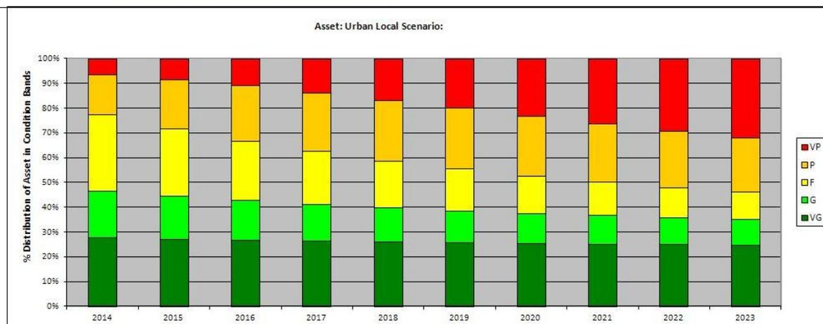
2.7 The above graph is part of the toolkit output associated with maintaining the present level of investment. The Urban Local Roads have been chosen to show the deterioration model as they represent 85% of the carriageway network length.
