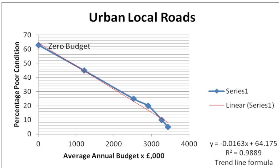
2.5 The series of graphs above indicate trends identified by using the new Life Cycle Planning toolkit provided by HMEP. The graphs enable the reader to see the average annual budget required to attain an overall highway condition. The lines are based on a 10 year planning cycle, therefore the graphs are showing what the percentage of poor or very poor condition roads will be present at the end of the 10 year period.
