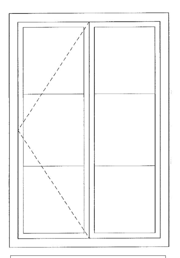
This plan is drawn to scale 1:10. On the plan the window is 9.2 cm in width by 13.3 cm in height. This means that the window would measure 92 cm in width by 133 cm in height in real life (i.e. exactly 10 times larger than on the plan)
