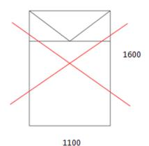
This plan cannot be accepted because the window frame width is not shown (a frame cannot be presented as a single line) and although measurements are shown it has not been drawn to an identified scale.
