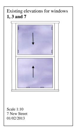
Where the details apply to more than one window (i.e. all relevant sizes are the same) then plans can refer to more than one window in the schedule, so long as it is clear which windows they apply to.
