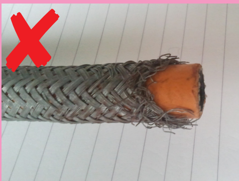
The braided hose is frayed.
