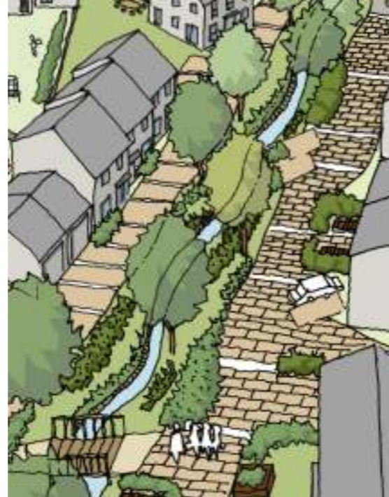
Homezone street with swale
