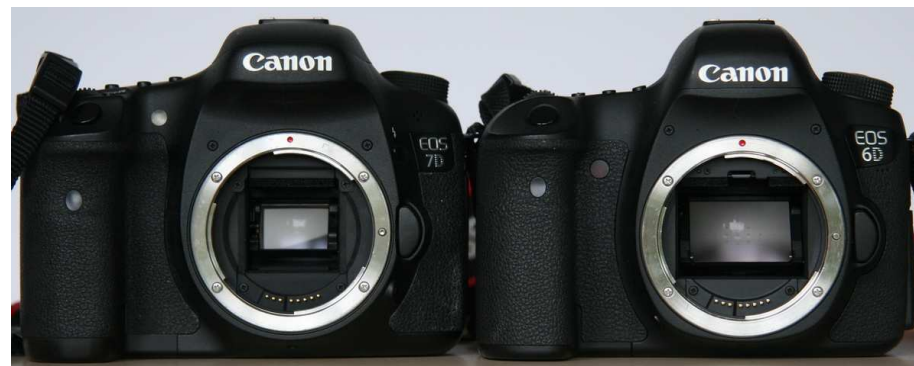
Fig A1.1 Illustration of Cropped-frame and Full-Frame Sensors (FFS): Canon 7D (cropped APS-C, left) and 6D (full-frame, right)
