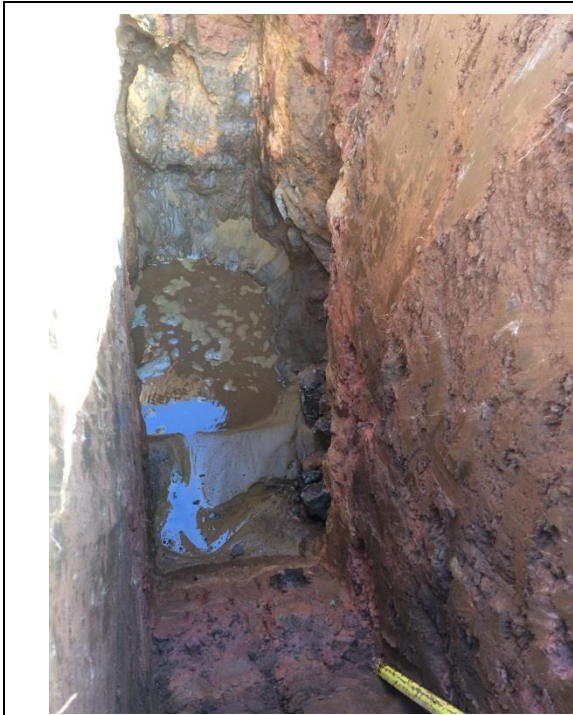
Plate 5 – TP3 showing the water running into a fissure in the bottom right hand corner
