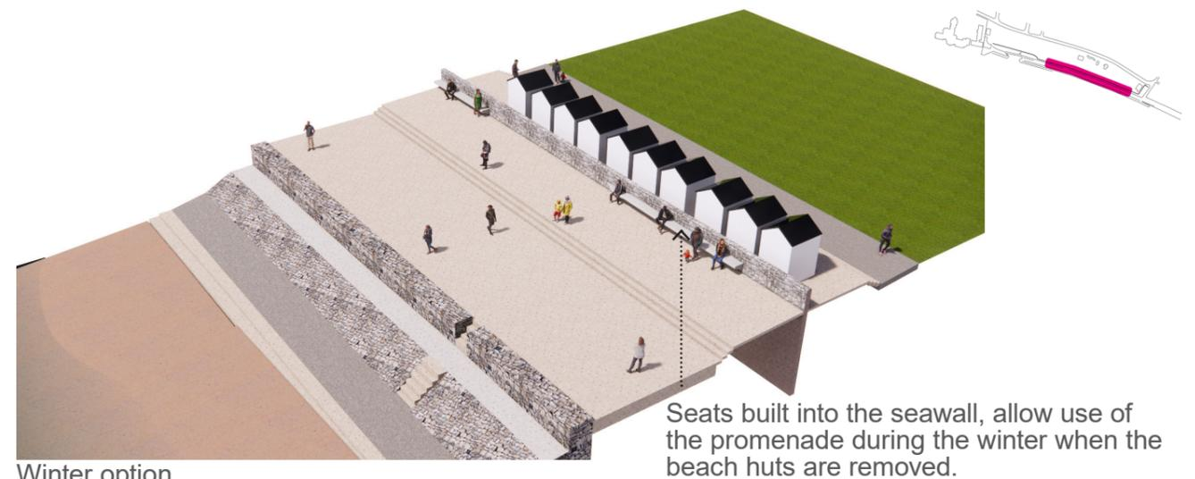
The existing shelters would be placed on buildouts along the raised plinth to simplify the alignment of the flood wall. The existing shelters could be refurbished, or new shelters provided. Ramped access would need to be incorporated to ensure that they are available for everyone.
