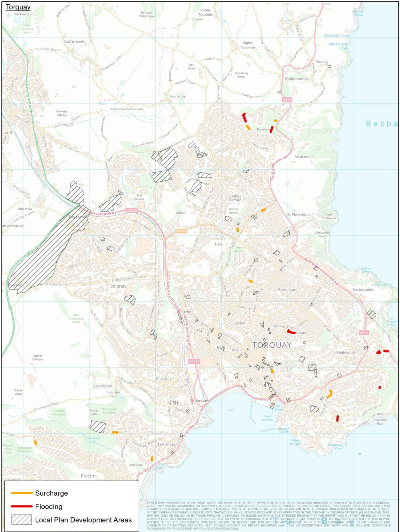
Broad locations of sewer flooding and areas excavated by additional pressure on the system based on M30-120 event model with development and creep Contains South West Water Ltd data. Contains Ordnance Survey data © Crown copyright and database right 2014
