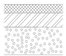
30mm thickness medium graded or dense Bitumen Macadam Surface Course with 6mm coarse aggregate min P.S.V. of 55
