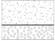
100mm Concrete Class 30 / 20 Aggregate to have a minimum P.S.V. of 55. Surface must be brush finished
